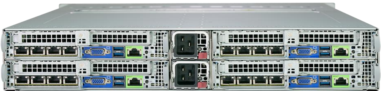
Figure 1. Rear View of 2U BigTwin Server System Showing 4 Hot-swap DP Nodes and 2 Redundant Power Supplies
