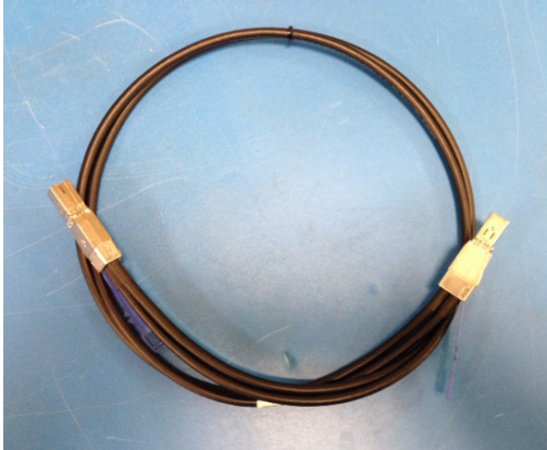
Figure 3-12. External Mini-SAS HD to External Mini-SAS HD Cable
