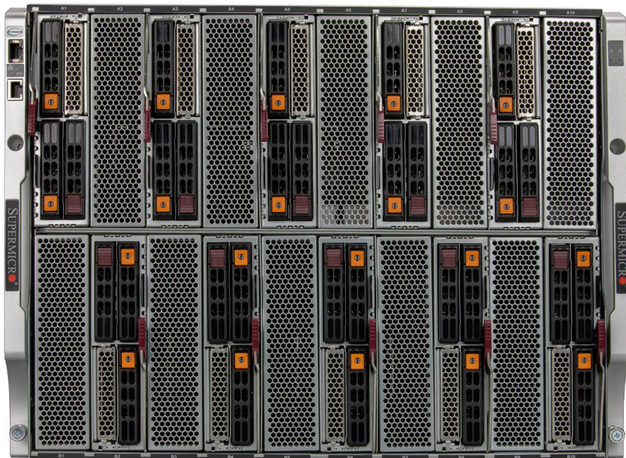
Figure 3-3. Installing Ten Half-Height, Double-Width Blades
