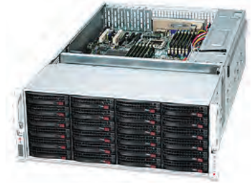
4U Storage HW SAS3 controller, Storage Expandable
