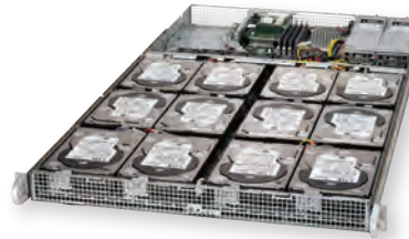
12-bay SoC Storage CDN, Warm Storage, Web/Database Server
