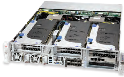
Front I/O, DC Power Optimized for 5G and Telco
