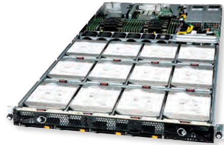
MegaDC - 1U Storage Top-loading Storage Featuring the New Internal Drawer Design
