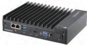
Extended Temperature Fanless IoT Gateway/Server
