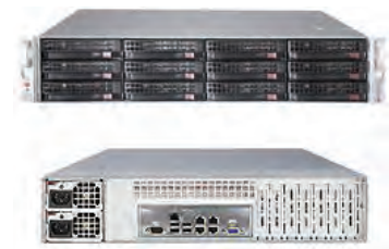
2U Storage SAS3 HW RAID controller Storage Expandable
