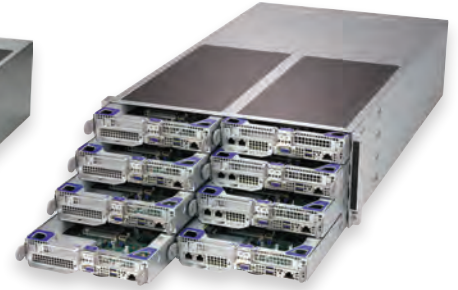
X11 FatTwin™ DP Intel® Xeon® Scalable processors, 2x 3.5" SSD/HDD per node
