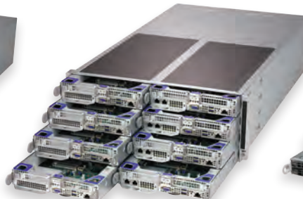
X11 FatTwin™ DP Intel® Xeon® Scalable processors with 2-4x 2.5" SSD/HDD per node
