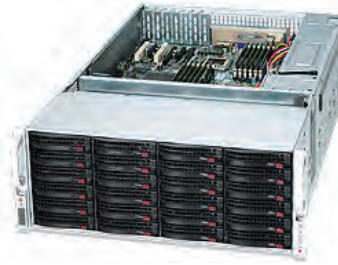
4U Storage HW SAS3 controller, Storage Expandable
