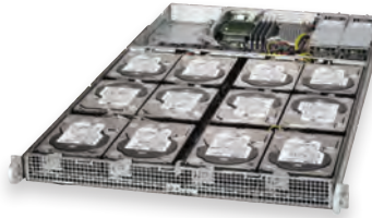
High-Density Cold Storage 12x 3.5 HDDs in 1U
