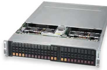
X11 BigTwin™ Dual DP Nodes, 24 Hybrid SAS3/NVMe Drive Bays
