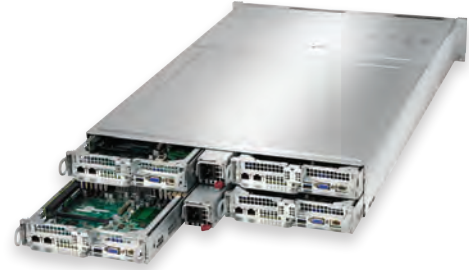
2U BigTwin™ 4 hot swappable nodes in 2U, Redundant Titanium Power
