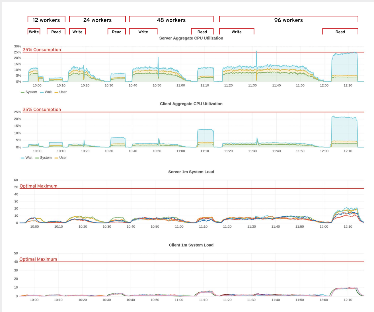
Figure 42. Figure 42. Server and client CPU and system load for 128GB files on a distributed-replicated volume on RAID 6 bricks.
