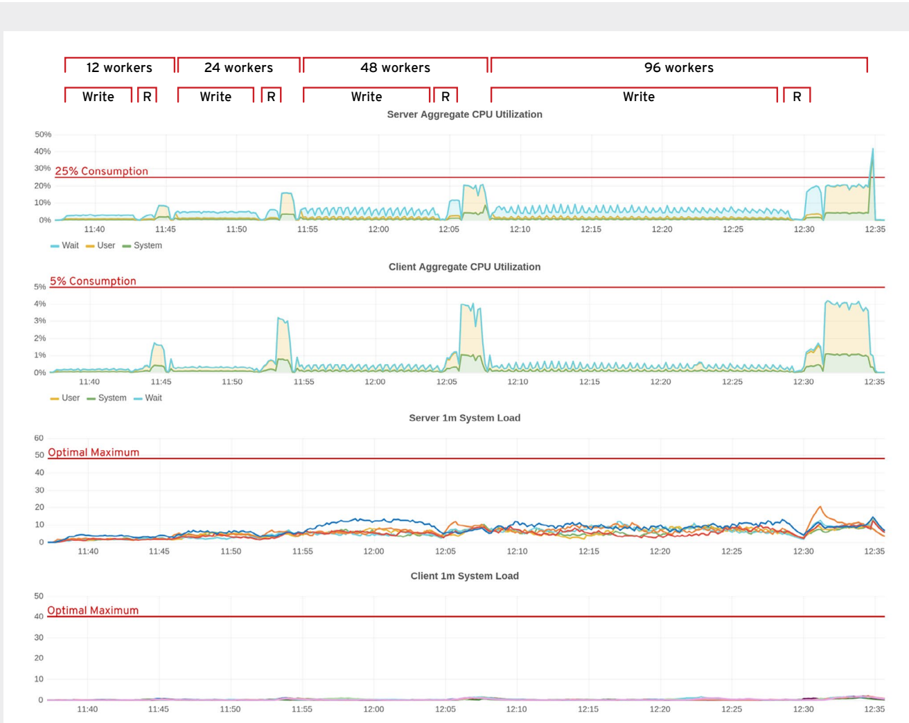
Figure 52. Server and client aggregate CPU utilization and system load remain well below optimum maximum levels.
