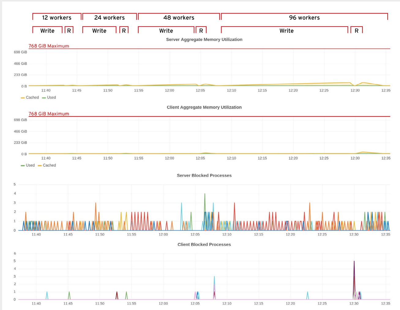
Figure 53. Memory utilization and blocked processes remained low for both servers and clients.
