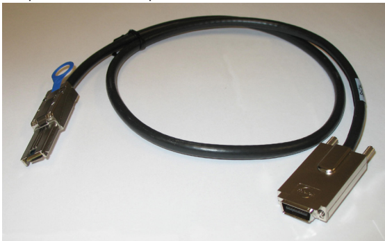
Figure E-22. External Cable (CBL-0166L)
