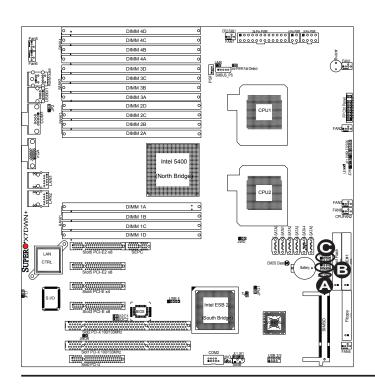
A. Compact Flash PWR B. SGPIO Header#1 C. SGPIO Header#2
