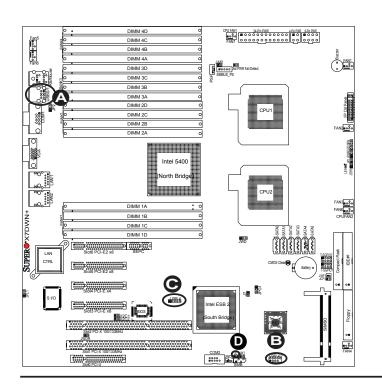
A. Backpanel USB 0/1 B. Front Panel USB 2/3 C. Front Panel USB 4
