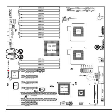
A. GLAN Port1 LEDs B. GLAN Port2 LEDs C. Onboard Power LED
