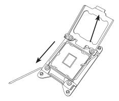
5. Using your thumb and index finger, hold the CPU by its edges. Align the CPU keys, which are semicircle notches, against the socket keys.
