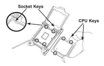
6. Once they are aligned, carefully lower the CPU straight down into the socket. Do not drop the CPU on the socket or move the CPU horizontally or vertically. Do not rub the CPU against the surface or against any of the socket pins to avoid damaging the CPU or the socket.
