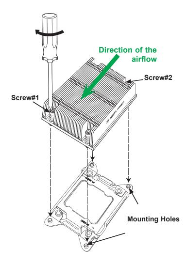
Note: For optimal airflow, please follow your chassis airflow direction to correctly install the CPU heatsink. Graphic drawings included in this manual are for reference only. They might look different from the components installed in your system.
