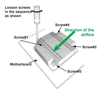
Notes: 1.) For optimized airflow, please follow your chassis airflow direction to properly install the heatsink. 2.) Graphics shown in this manual are for reference only. They may or may not look the same as the components installed in your system.
