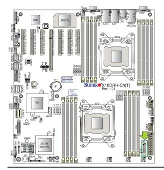
A. Reset Button B. PWR Button BPower Button Ground AReset Button Ground Power Fail LED 3.3V OH/Fan Fail/ 0 UID LED PWR Fail LED) NIC2 Activity LED NIC2 Link LED NIC1 Activity LED NIC1 Link LED UID Switch HDD LED FP PWRLED 3.3 V  $\circ$ 0 0 x Ground NMI 20
