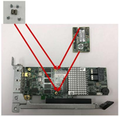
Figure 3-3. Install TFM module onto RAID add-on module
