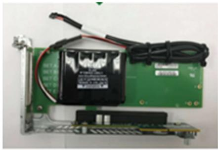
Figure 3-2. Install battery pack and wrap power cable
