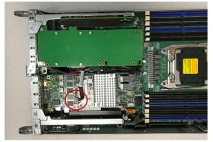
Figure 3-4. Connect power cable to the TFM module
