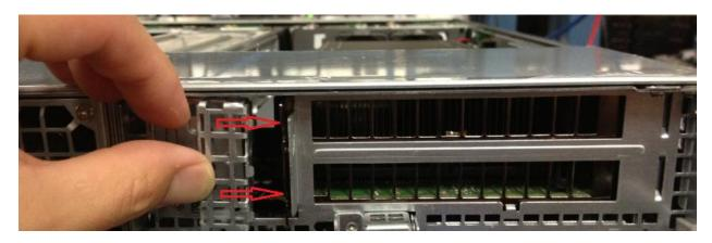
8. Secure the GPU with the 2-mm screw as indicated.
