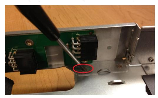
4. Secure the MB tray assembly and power adaptor card & riser card bracket firmly secured together.
