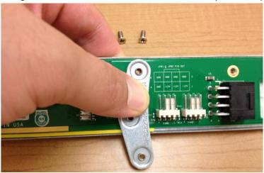
3. Hold the bracket and the sheet metal and, fasten them together with the screws.
