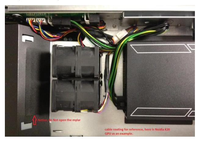
Completed the GPU kit with GPU correctly installed.
