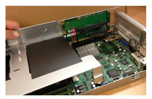
$6. \quad \text{Secure the motherboard tray support bracket with two 3mm screws.} \\$
