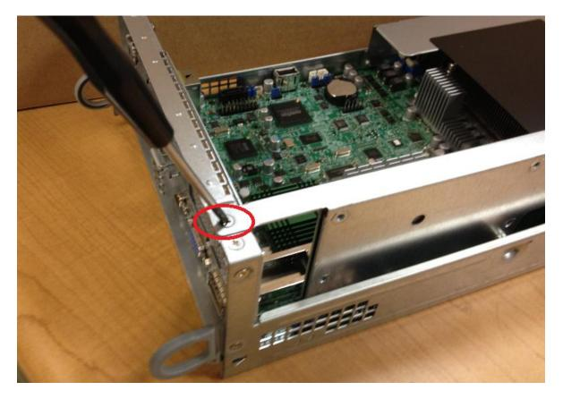
**⑤** Confirm four screws are secured on the bracket.
