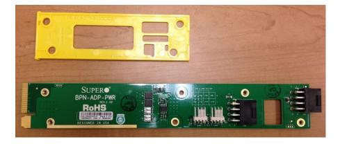
3. Place the plate on the back of the power adaptor card.
