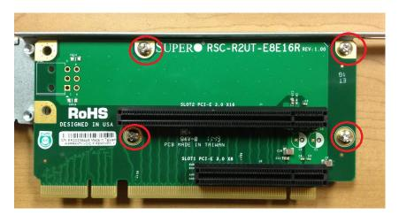
3. Confirm that six screws are now attached to the support bracket.
