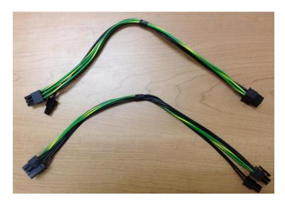
2. Insert the 8-pin connector into JPW1.
