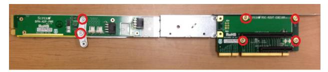
Attaching the Motherboard tray support bracket to the power adaptor & riser card support bracket:
