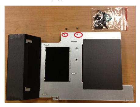
2. Secure the complete bracket of power adaptor and riser card bracket assembly to the MB tray support bracket with the two screws.
