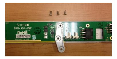
2. Align the holes on the bracket with those on the power adaptor card.
