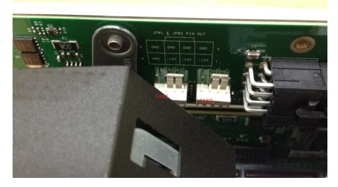
5. Connect FAN1 and FAN2 to the FAN1 and FAN2 connectors on the power adaptor card.
