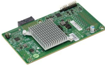
Figure 4-8. AOC-OPA-WFR Mezzanine OPA Card
