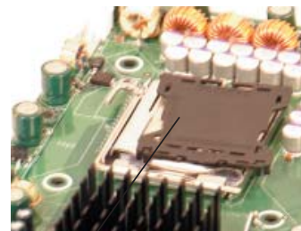
Plastic cap is released from the load plate when the CPU is properly installed.
