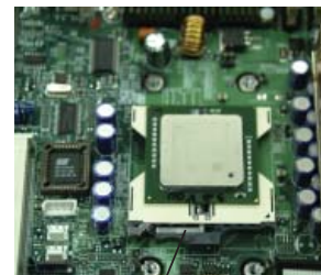
Socket lever in the locked position
