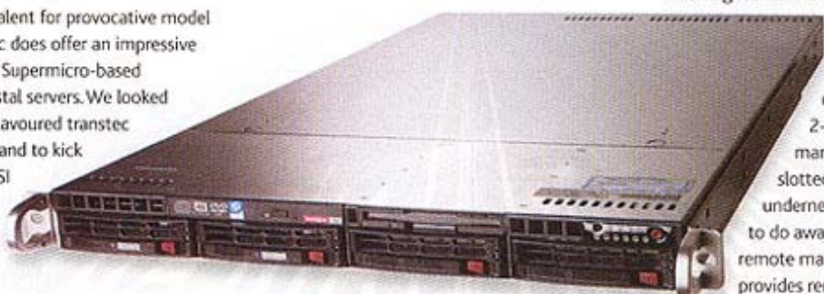
Hot-swap power supplies make their first appearance in a Supermicro-based rack server.
