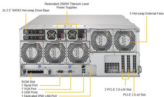
**Figure 5.** SuperStorage Top-Loading 45- or 60-Bay Storage Server (Rear View)
