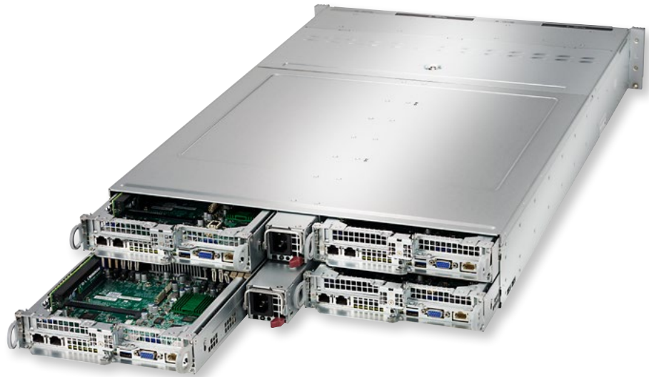
Figure 1. Rear View of 2U BigTwin Server System Showing 4 Hot-swap DP Nodes and 2 Redundant Power Supplies
