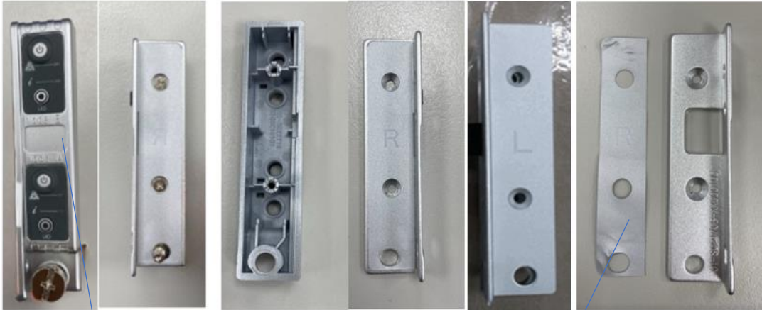
Remove control panel screw (R and L) from chassis
