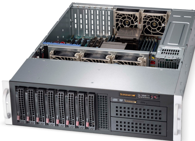
Figure 9. Supermicro SuperServer (SYS-6037R-72RFT)
