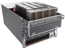
The NVIDIA HGX H100 GPUs increases training and inference performance compared to any other GPU in the market. The Supermicro SYS-821GE-TNHR that Genesis Cloud is using for its AI cloud includes:
