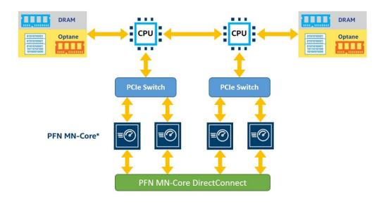
**Block diagram of PFN solution**
