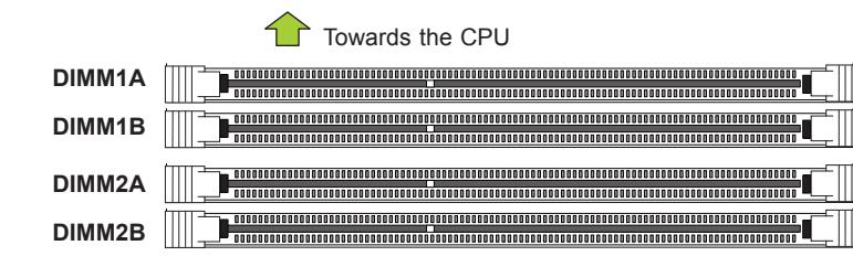
**Note:** Please populate the memory slots in the following order for optimal results: DIMM1A, DIMM2A, DIMM1B, DIMM2B.
