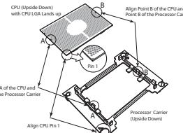
2 To form the processor heatsink module (PHM), mount the processor carrier assembly onto the heatsink and snap into place.
