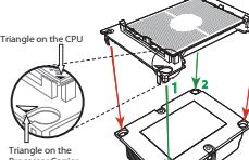
3 After assembling the PHM, mount it onto the CPU socket of the motherboard. Use a T-30 Torx-bit screwdriver to gradually install four screws into the mounting holes from #1-4.
