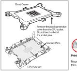
emoving the Processor Heatsink Module (PHM) from the Motherboard Remove the dust cover from the CPU socket, exposing he socket and socket pins as shown on the illustration Note: Do not touch the socket pins to avoid dama
