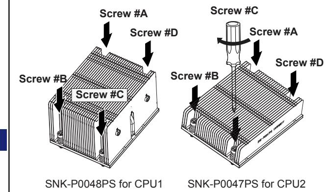
1. Place heatsink on top of installed CPU
