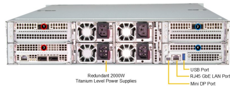
(Rear View – System)
