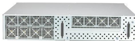
**System Cooling** Fans: Up to 12x 4cm heavy duty fans with optimal fan speed control 40x40x56mm Fan(s)
