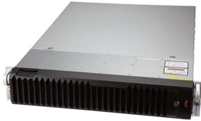
Equipment that is certified to be NEBS Level 3-compliant must undergo a series of tests that are conducted and confirmed by a certified Third Party Lab (TPL). The tests for NEBS Level 3 are based on Telcordia NEBS documents SR-3580 and GR-63, which ensure the equipment meets certain physical protection requirements, and GR-1089 which ensures the equipment meets specific requirements for electromagnetic compatibility and electrical safety.
