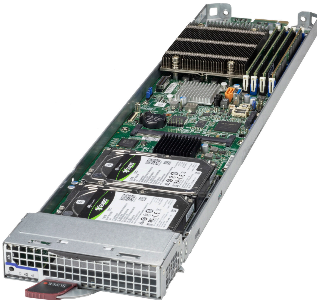
Figure 2-3. Storage Drive Installed
