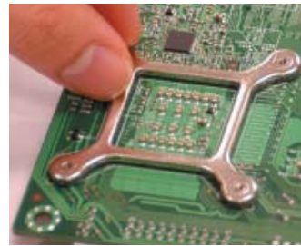
Heatsink bracket properly seated on the MB
