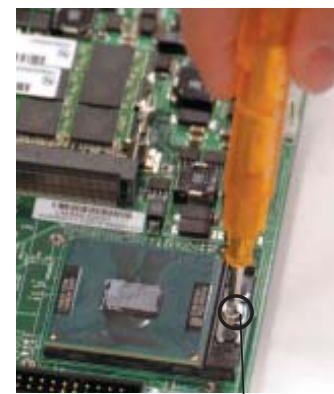
Using a Flathead screwdriver, turn clockwise to lock the CPU
