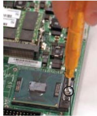
Using a Flathead screwdriver, turn counter-clockwise to unlock the CPU
