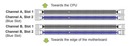
The X10SLD-F/-HF supports up to 32GB of Unbuffered (UDIMM) DDR3 ECC 1600/1333/1066 MHz in 4 memory slots. Populating these DIMM modules with a pair of memory modules of the same type and same size will result in interleaved memory, which will improve memory performance. Please refer to the table below:
