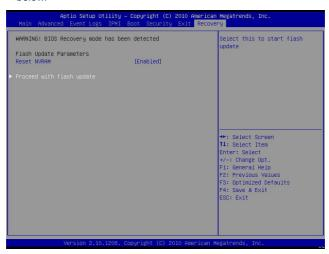
When the screen as shown above displays, using the arrow key, select the item- "Proceed with flash update" and press the <Enter> key. You will see the progress of BIOS Recovery as shown in the screen below.
