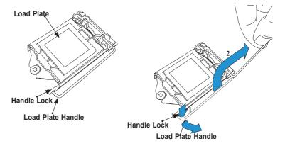
Once the load plate is open, use your thumb and your index finger to hold the CPU at the north center edge and the south center edge of the CPU.
