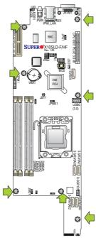
**Caution:** 1) To avoid damaging the motherboard and its components, please do not use a force greater than 8 lb/inch on each mounting screw during motherboard installation. 2) Some components are very close to the mounting holes. Please take precautionary measures to avoid damaging these components when installing the motherboard to the chassis.
