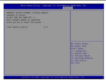
After the process of BIOS Recovery is complete, press any key to reboot the system.
