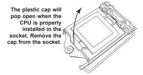
**Warning:** You can install the CPU inside the socket only in one direction. Make sure that it is properly inserted into the CPU socket before closing the load plate. If it doesn't close properly, do not force it, as that may damage your CPU. Instead, open the load plate again and check whether the CPU is properly aligned and securely seated inside the socket.
