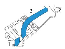
2. Gently lift the load lever to open the load plate. Remove the plastic cap.
