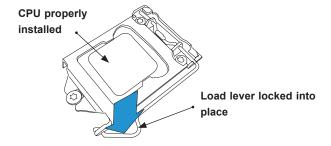
**Note:** You can only install the CPU inside the socket in one direction. Make sure that it is properly inserted into the CPU socket before closing the load plate. If it doesn't close properly, do not force it as it may damage your CPU. Instead, open the load plate again and double-check that the CPU is aligned properly.
