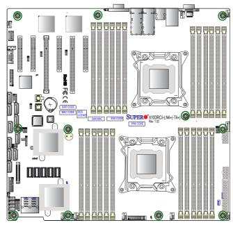
**Caution:** 1) To avoid damaging the motherboard and its components, please do not use a force greater than 8 lb/inch on each mounting screw during motherboard installation. 2) Some components are very close to the mounting holes. Please take precautionary measures to prevent damage to these components when installing the motherboard to the chassis.
