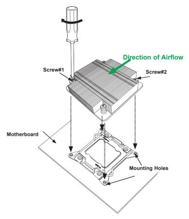
Note: For optimized airflow, please follow your chassis airflow direction to properly install the heatsink. Graphics and drawings included in this manual are for reference only. They might look different from the components installed in your system.
