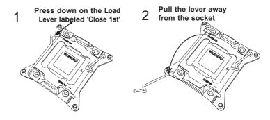
With the lever labelled 'Close 1st' fully retracted, gently push down on the lever labelled 'Open 1st' to open the load plate. Lift the load plate to open it completely.
