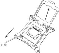
5. Using your thumb and index finger, hold the CPU on its edges. Align the CPU keys, which are semi-circle cutouts, against the socket keys.
