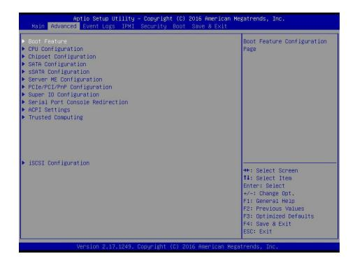
**Warning**: Take caution when changing the Advanced settings. An incorrect value, a very high DRAM frequency, or an incorrect DRAM timing setting may make the system unstable. When this occurs, revert to the default to the manufacture default settings.
