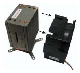
Unscrew the heatsink screws from the motherboard in a diagonal sequence, as shown in the illustration to the right.
