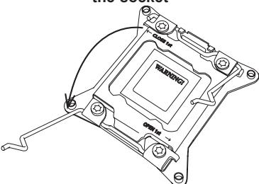
3. With the lever labeled 'Close 1st' fully retracted, gently push down on the 'Open 1st' lever to open the load plate. Lift the load plate to open it completely.
