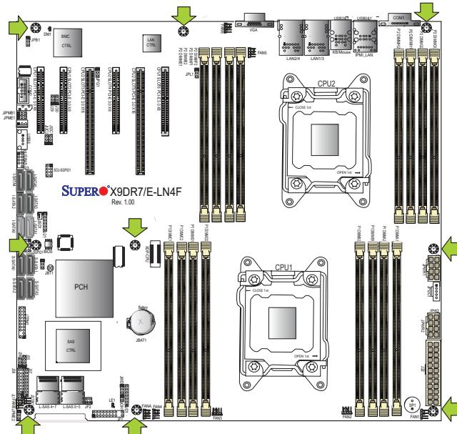
**Warning:** 1) To avoid damaging the motherboard and its components, please do not use a force greater than 8 lb/inch on each mounting screw during motherboard installation. 2) Some components are very close to the mounting holes. Please take precautionary measures to prevent damage to these components when installing the motherboard to the chassis.
