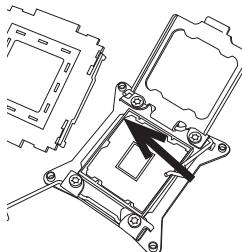
2. Once they are aligned, carefully lower the CPU straight down into the socket. (Do not drop the CPU on the socket. Do not move the CPU horizontally or vertically. Do not rub the CPU against the surface or against any pins of the socket to avoid damaging the CPU or the socket.)
