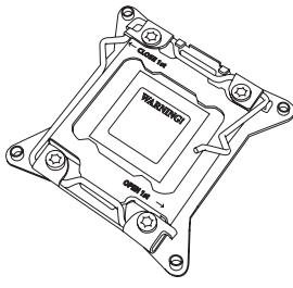
2. Press the second load lever labeled 'Close 1st' to release the load plate that covers the CPU socket from its locking position.
