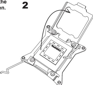
1. Use your index finger and your thumb to loosen the lever and open the load plate. Align Pin1 of the CPU with Pin 1 of the CPU Socket.
