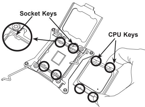
3. With the CPU inside the socket, inspect the four corners of the CPU to make sure that the CPU is properly installed.
