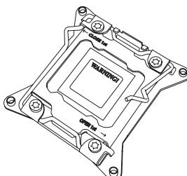
2. Press the second load lever labeled 'Close 1st' to release the load plate that covers the CPU socket from its locking position.
