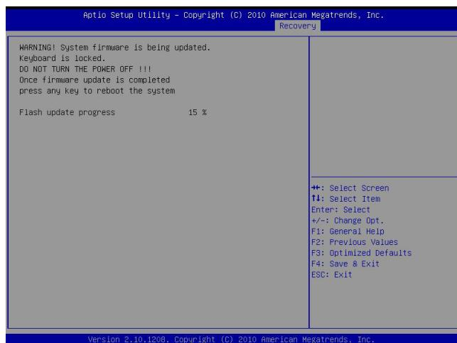
6. After the process of BIOS recovery is completed, press any key to reboot the system.
