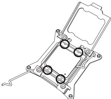
**Warning:** You can only install the CPU inside the socket in one direction. Make sure that it is properly inserted into the CPU socket before closing the load plate. If it doesn't close properly, do not force it as it may damage your CPU. Instead, open the load plate again and double-check that the CPU is aligned properly.
