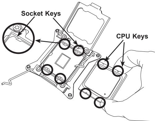
3. Once they are aligned, carefully lower the CPU straight down into the socket. (Do not drop the CPU on the socket. Do not move the CPU horizontally or vertically. Do not rub the CPU against the surface or against any pins of the socket to avoid damaging the CPU or the socket.)
