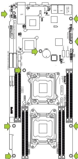
**Caution:** 1) To avoid damaging the motherboard and its components, please do not use a force greater than 8 lb/inch on each mounting screw during motherboard installation. 2) Some components are very close to the mounting holes. Please take precautionary measures to prevent damage to these components when installing the motherboard to the chassis.
