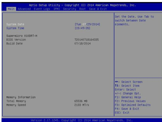
When you first enter the AMI BIOS Setup utility, you will enter the Main setup screen. You can always return to the Main setup screen by selecting the Main tab on the top of the screen. The Main BIOS Setup screen is shown below.
