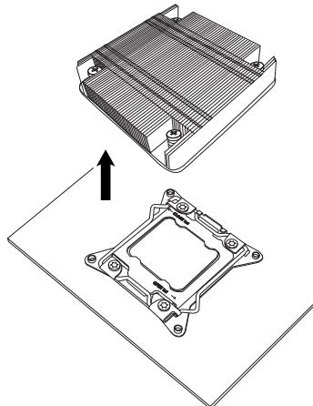
4. Once the heatsink is loosened, remove it from the motherboard.
