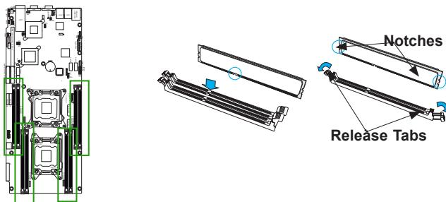
3. Align the key of the DIMM module with the receptive point on the memory slot.
