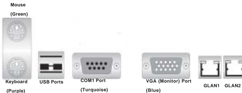
Figure 2-3. I/O Port Locations and Definitions
