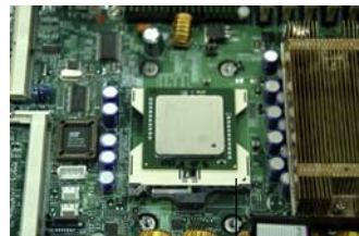
Socket lever in the locking Position
