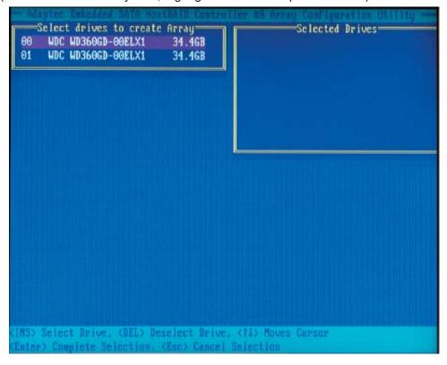
5. Press Enter when both disks for the new array are selected. The Array Properties menu displays (as the screen shown below).
