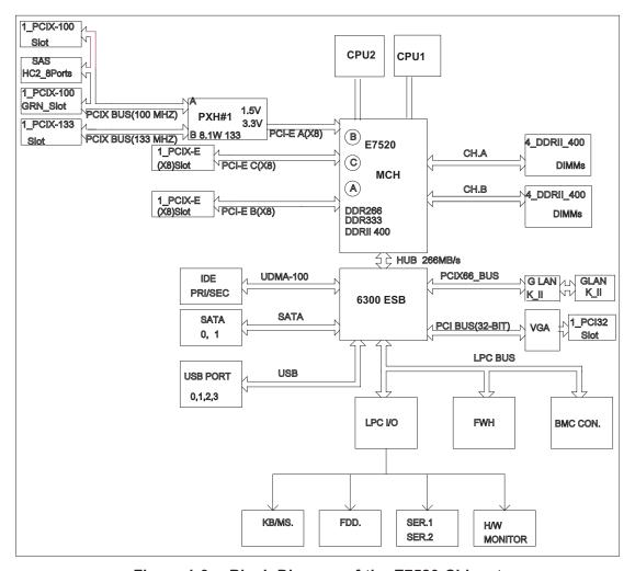
Figure 1-9. Block Diagram of the E7520 Chipset
