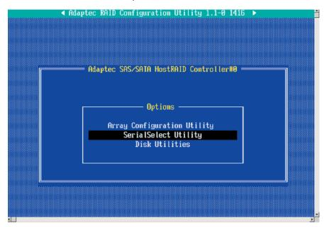
2. Use the arrow keys to select "SerialSelect Utility" and press <Enter> to access the Controller Configuration submenu:
