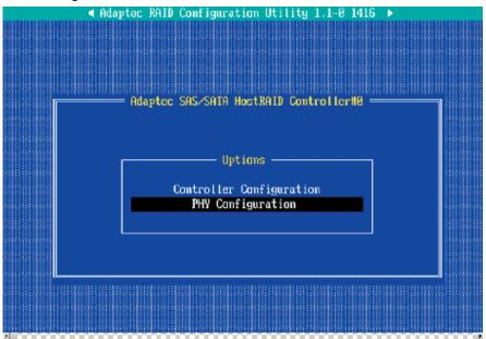
3. Select "Physical Configuration" and press <Enter> to access SAS Device Configuration submenu as shown below:
