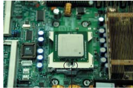
Socket lever in the locking Position
