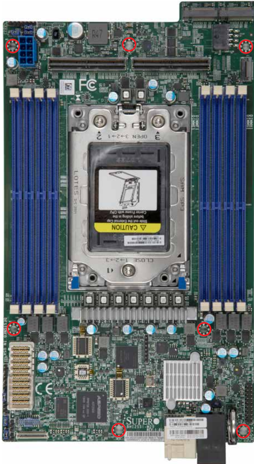
Figure 2-1. Motherboard Mounting Holes
