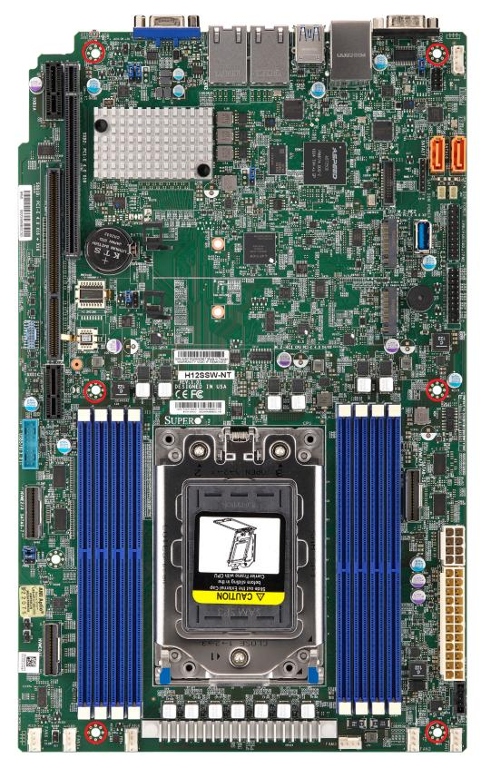
Figure 2-1. Motherboard Mounting Holes
