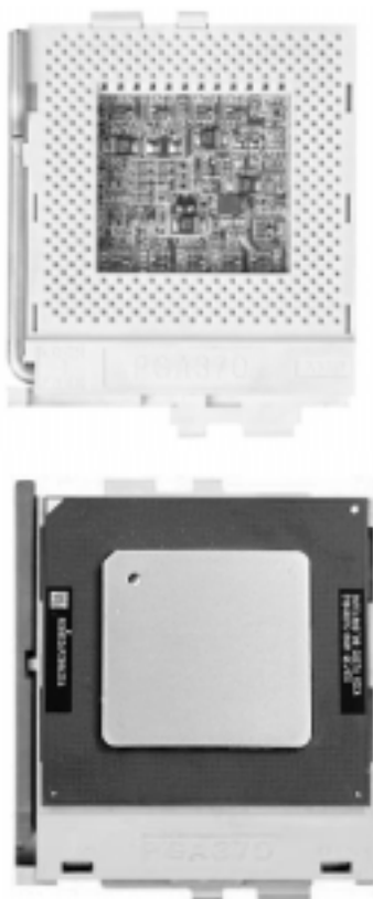
Figure 2-3. FCPGA Socket: Empty and with Processor Installed (low power Pentium III shown)
