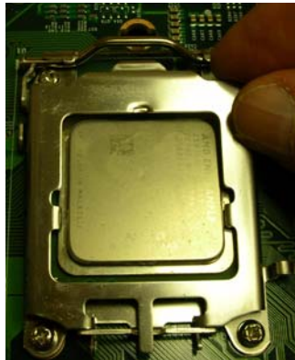
Figure 2-4. Inspecting the CPU Installation
