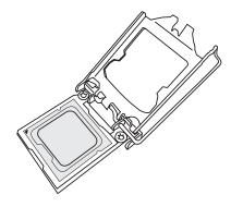
5. Close the load plate, then gently push down the load lever into its locking position.
