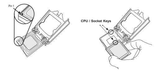
4. Carefully lower the CPU straight down into the socket. Do not drop the CPU on the socket, or move it horizontally or vertically to avoid damaging the CPU or socket. Inspect the four corners of the CPU to make sure that the CPU is properly installed.
