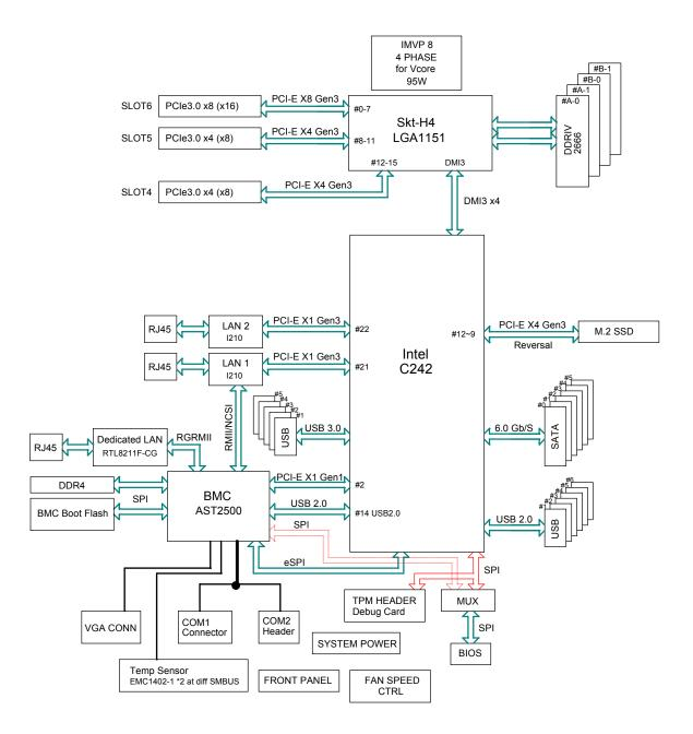
Figure 1-3. C242 System Block Diagram
