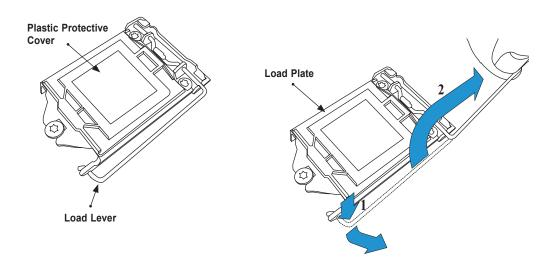
2. Gently lift the load lever to open the load plate. Remove the plastic protective cover. Do not touch the CPU socket contacts.
