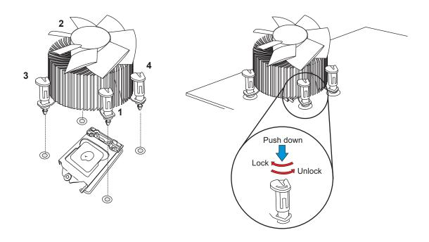
7. Once all four fasteners are secured, connect the heatsink fan wire connector to the CPU fan header.
