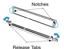
Press both notches straight down into the memory slot.
