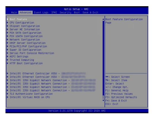
**Warning**: Take caution when changing the Advanced settings. An incorrect value, a very high DRAM frequency, or an incorrect DRAM timing setting may make the system unstable. When this occurs, revert to default manufacturer settings.
