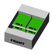
Figure 2-6: Motherboard Locations In the Chassis
