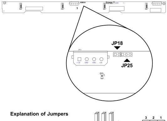
To modify the operation of the backplane, jumpers can be used to choose between optional settings. Jumpers create shorts
