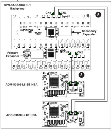
Figure 3-3. Backplane Cascading Configuration
