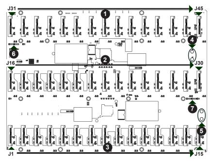
Figure 2-1. BPN-SAS3-946LEL1 Connector Side Components
