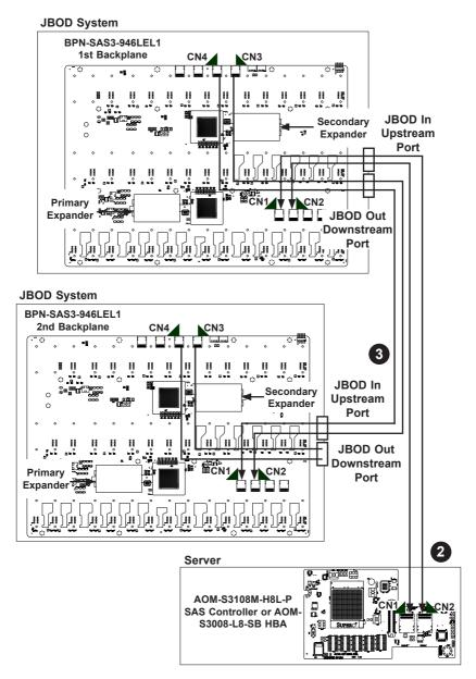
Figure 3-2. Backplane Cascading Configuration
