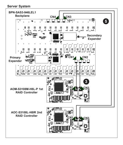
Figure 3-4. Backplane Cascading Configuration
