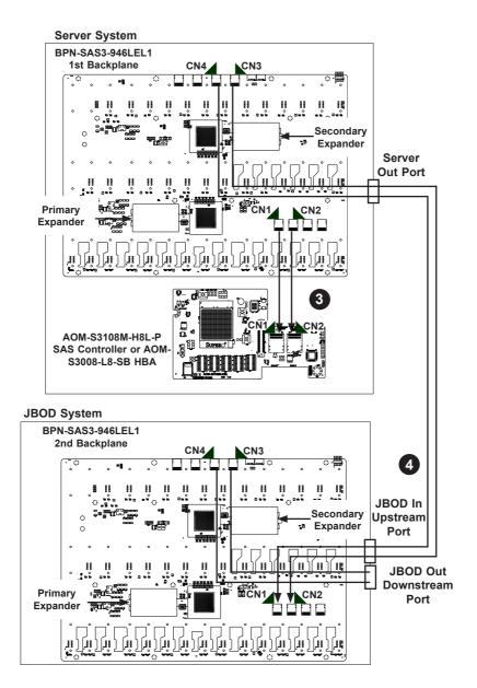
Figure 3-1. Backplane Cascading Configuration
