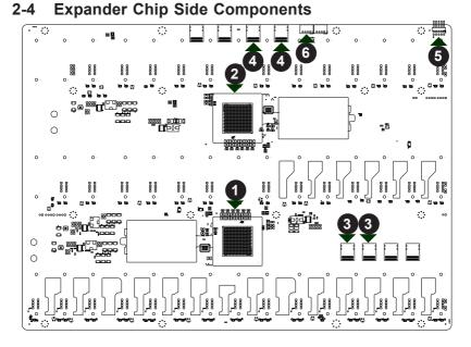
Figure 2-3. BPN-SAS3-946LEL1 Expander Chip Side Components
