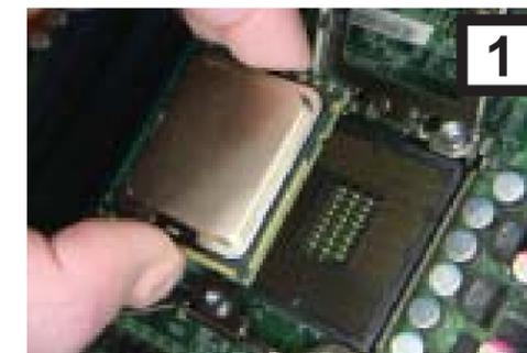
2. Locate Pin 1 of the CPU, which is marked with a gold triangle on the CPU. Locate Pin 1 of the socket, which is marked with a triangle on the socket or the motherboard.
