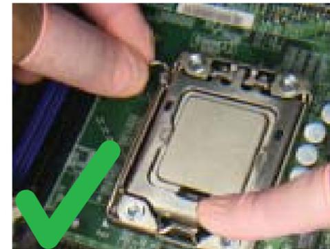
**14. Install and remove the CPU properly.**
