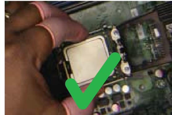
**6. Holding the center edges of the CPU, insert it straight down into the socket.**
