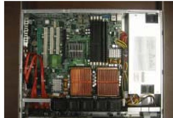
2. **Install the CPU/Heatsink after placing the motherboard in the chassis.**
