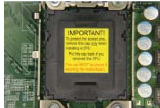
3. **Upon receiving a CPU, make sure that the plastic cap is in place. Inspect for bent pins.**
