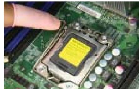
1. **Secure the motherboard with one hand and use another to unlock the load plate.**
